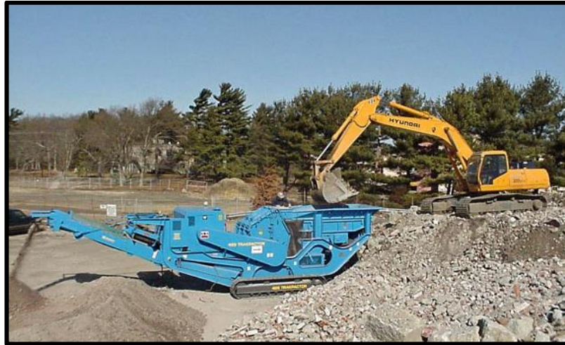
Figure 5-1: Simple recycled concrete aggregate crusher (Eagle Crushers, 2016)
