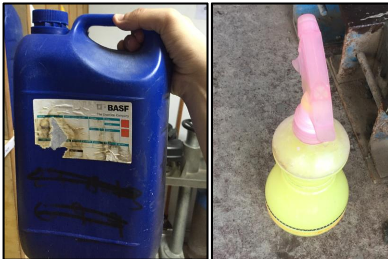
Figure 3-4: BASF MasterCure 181 was used as a curing compound. It was added to a sprayer to be sprayed over the finished surface of concrete
