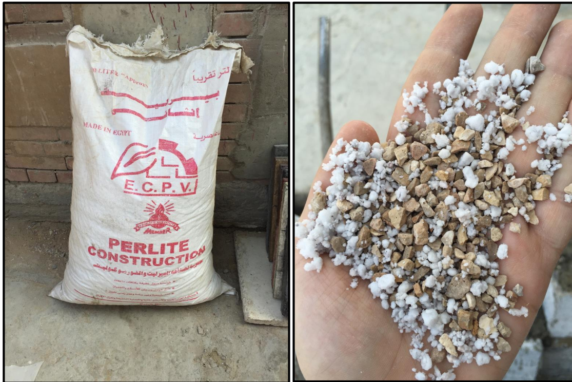
Figure 3-2: Structural Perlite bag and its grain size compared to crushed sand
