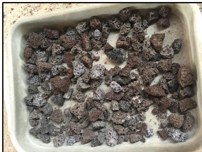
Figure 3-3: Pumice lightweight aggregates used
