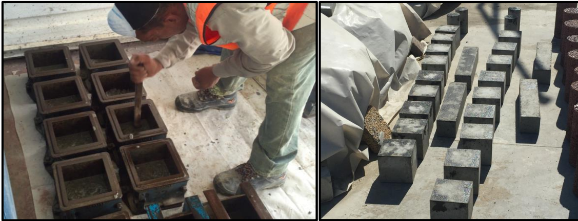
Figure 3-7: Placing and finishing of concrete specimens
